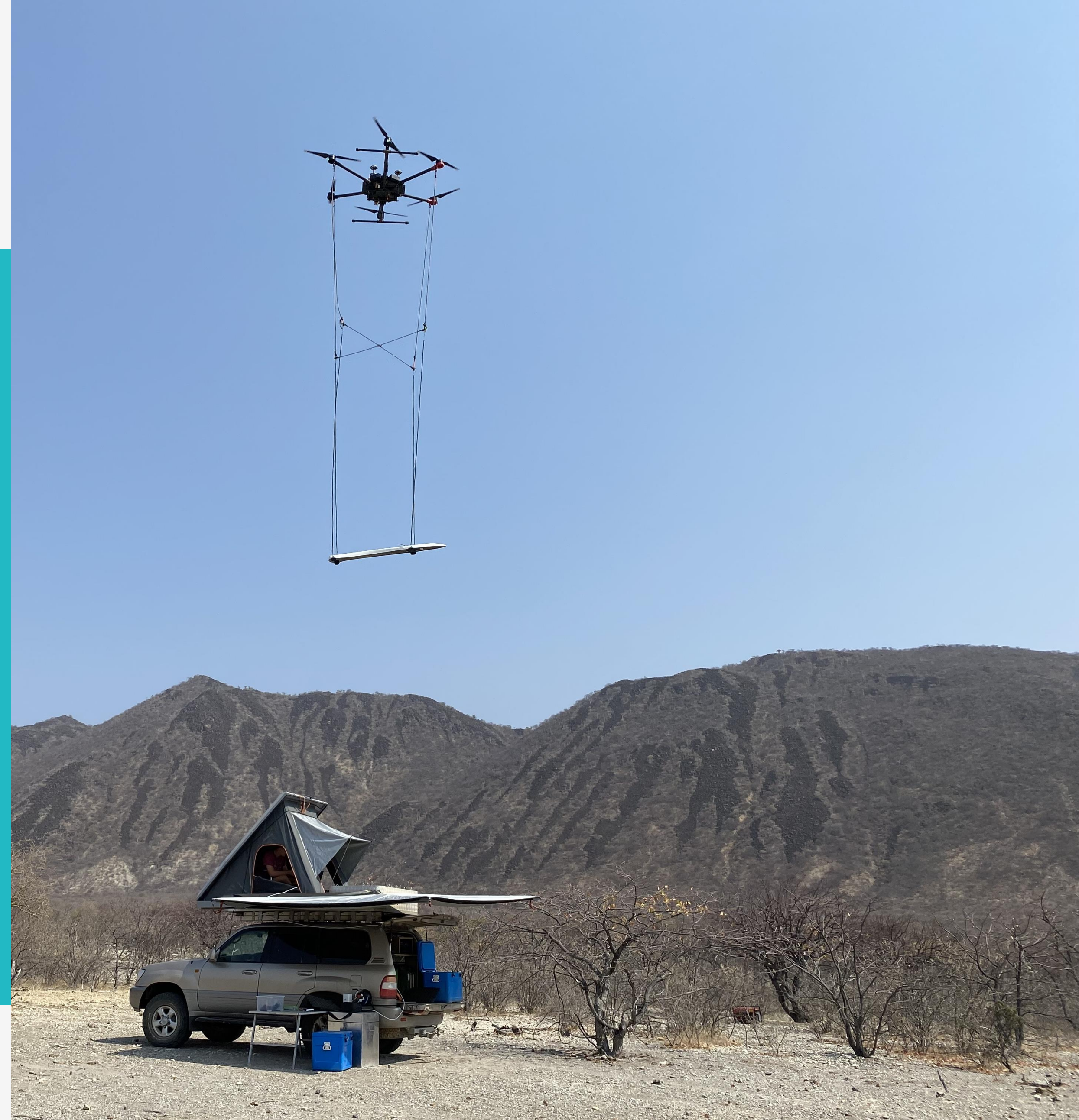
Magnetic sensor suspended beneath the drone
